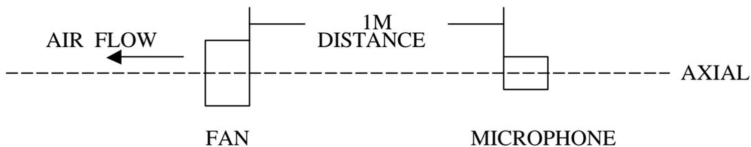
6-2. MEASUREMENT PERFORMED IN ANECHOIC TEST CHAMBER UNDER FREE AIR CONDITION.
